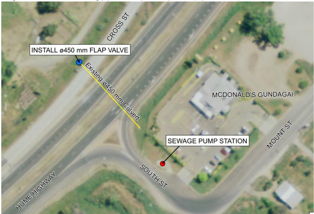
Diagram 7 Location of existing pipe and required flap valve (Option FM10)
